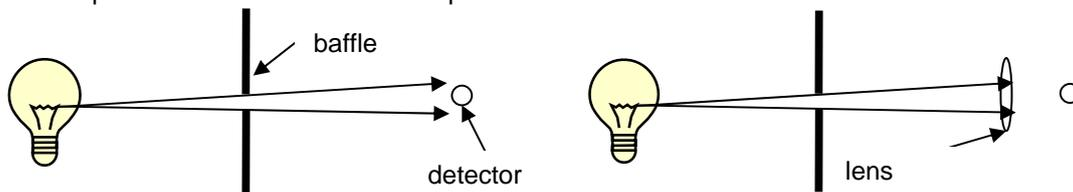
Figure 2, lamp with baffle, detector and lens
