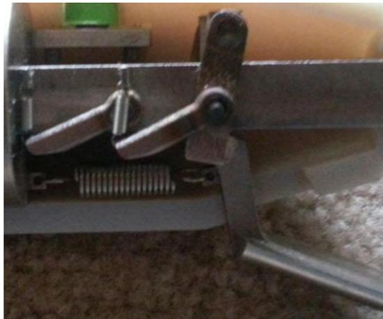
Figure 4.6: The ratcheting mechanism made up of a four bar crank slider configuration.
