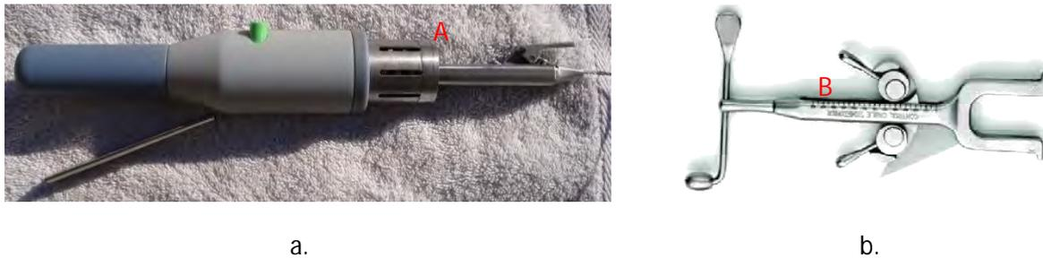
Figure 8.5: a) The new instrument's tension meter; b) The old instrument's tension meter.
