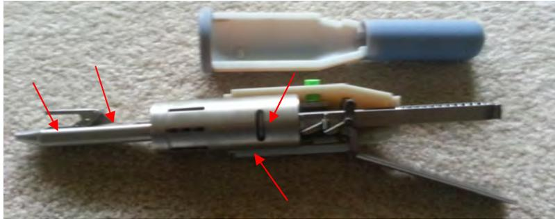
Figure 6.5: The areas of the instrument most likely to cause sterilization problems
