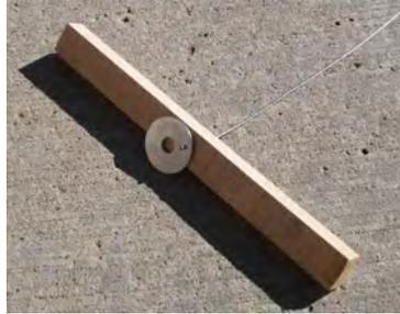
Figure 6.2: A close up picture of the parts used to support the weights used during the tests.
