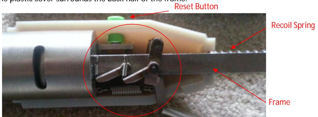
Figure 4.3: The assembly of the tension meter and the frame with the surrounding components.
