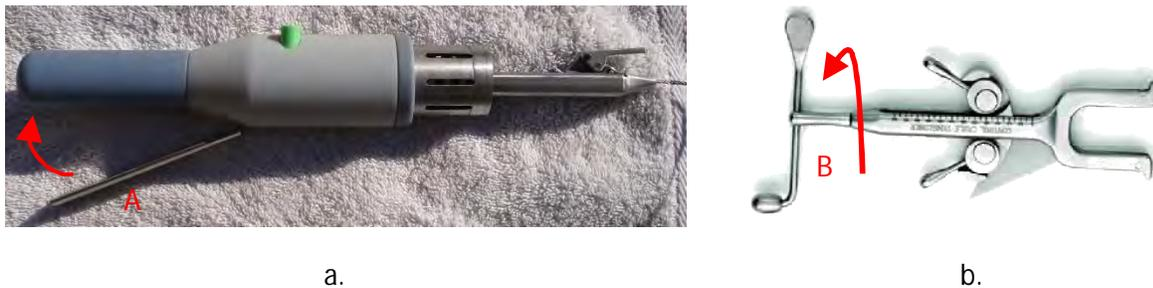
Figure 8.2: a) Tensioning the cable with the new instrument; b) Tensioning the cable with the old instrument.
