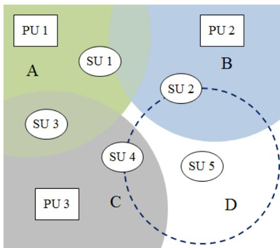
Fig. 5.3. Example CRN with three PU transmitters and five SUs; transmit radius of secondary user  $SU 5$  represented by dotted line.
