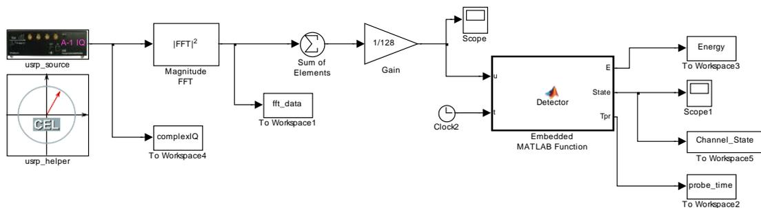
Fig. 6.1. Simulink-USRP implementation of an energy detector.
