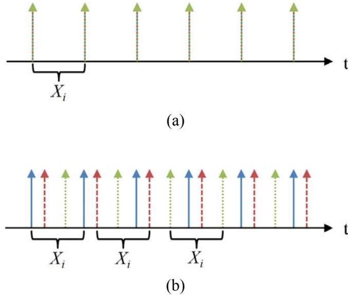
Fig. 7.1. Synchronized periodic spectrum probing (a) and independent periodic spectrum probing by three users (b).
