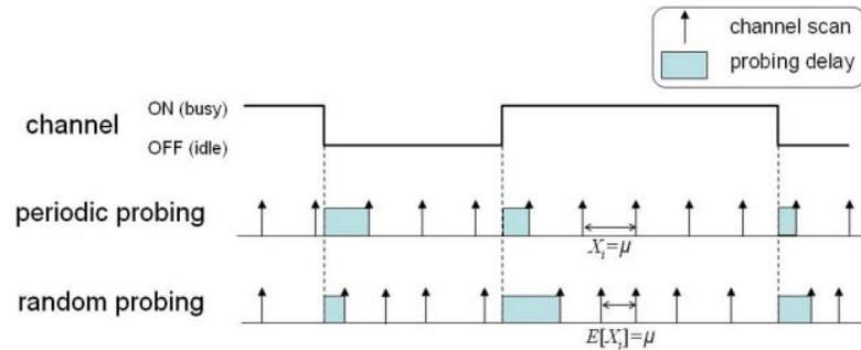
Fig. 7.2. Illustration of periodic and random probing methods.
