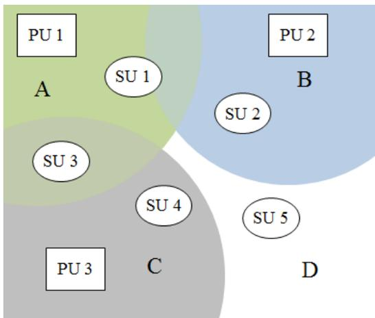
Fig. 5.2. Example CRN with three PU transmitters and five SUs;  $SU5$  is out of range of all PU transmitters.
