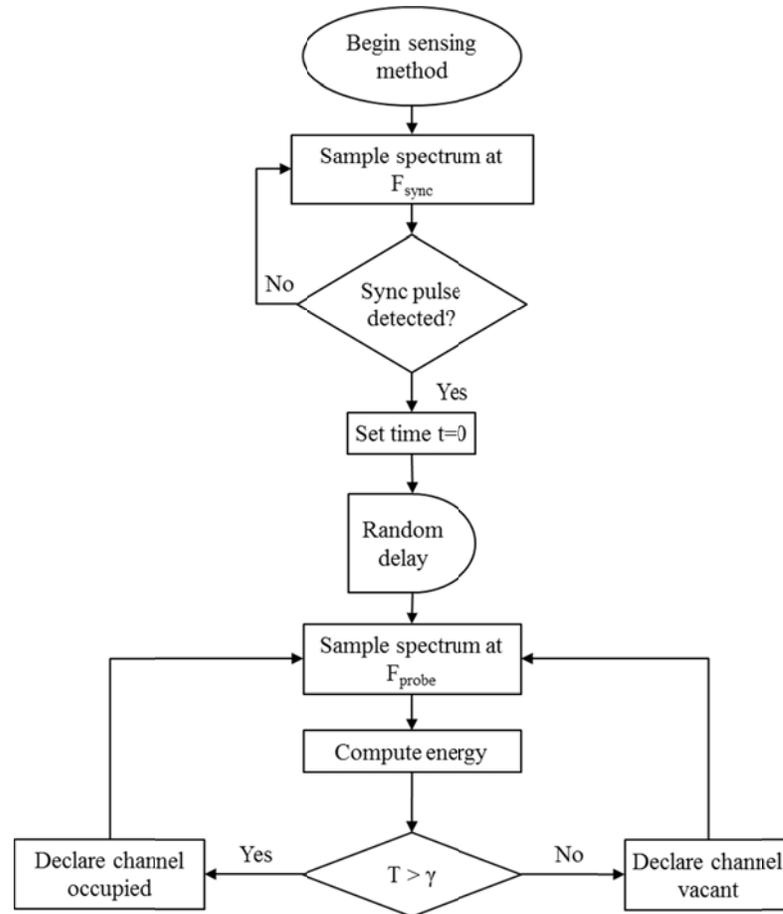
Fig. 8.3. Flowchart of Simulink-USRP energy detector process.
