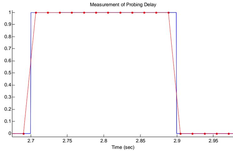
Fig. 7.4. Small probing delay, resulting in interference. Blue – actual channel state, Red – probed channel state. 0=vacant, 1=occupied.
