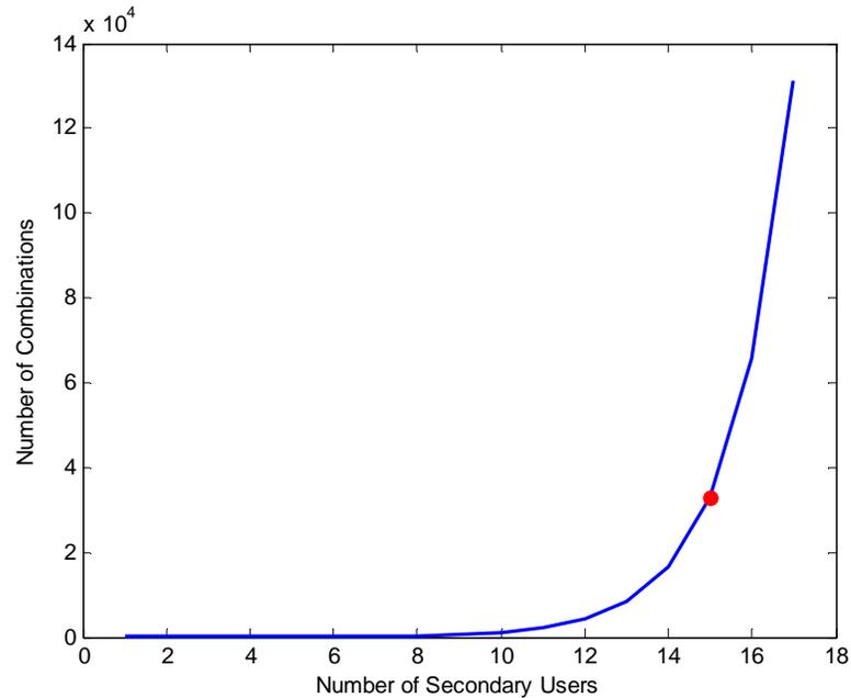
Fig. 9.16. Exponential growth of SU combinations required to compute, combinations of 15 SUs indicated.
