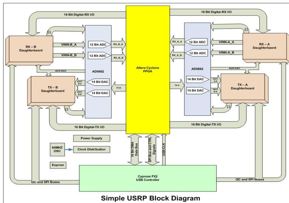
Fig. 1.1. USRP block diagram.
