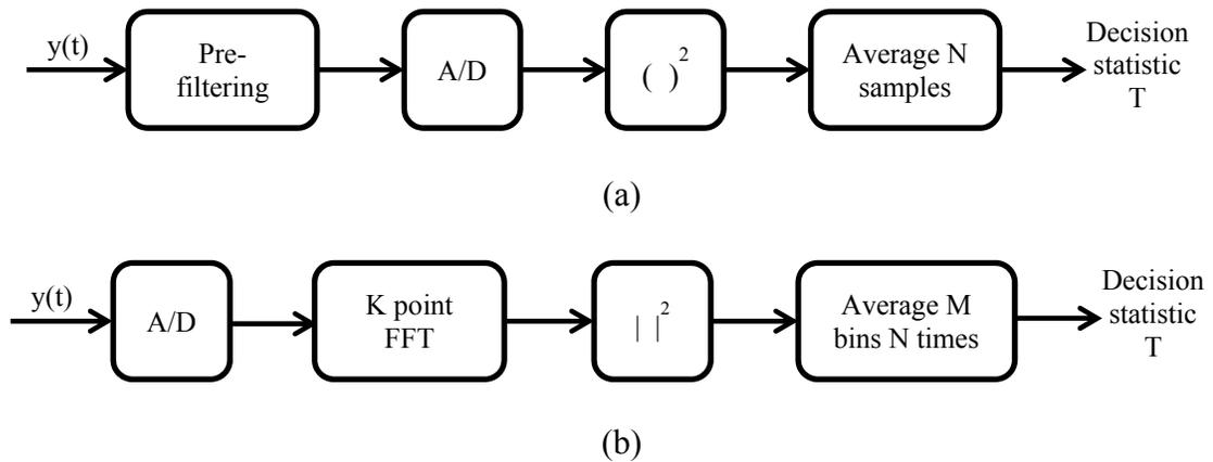
Fig. 5.1. Energy detection method (a) with an analog pre-filter and square-law device (b) with FFT magnitude squared and averaged.
