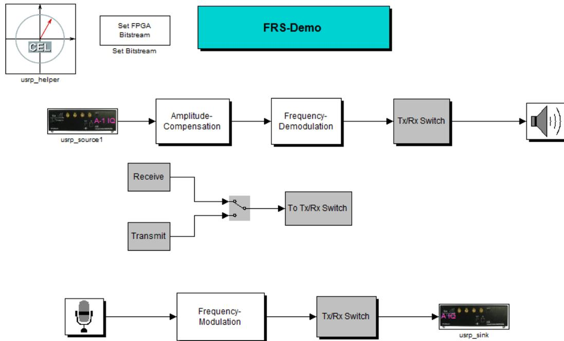
Fig. 3.3. Simulink-USRP demo application for building an FM half duplex transceiver.
