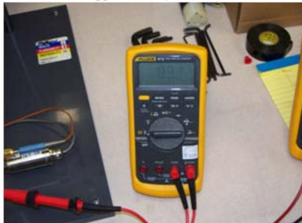
**Figure 18-Multi-Meter Reading at Approximately 90 Volts**
