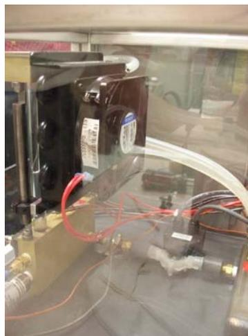
Figure 7: Tube Fin Condenser
