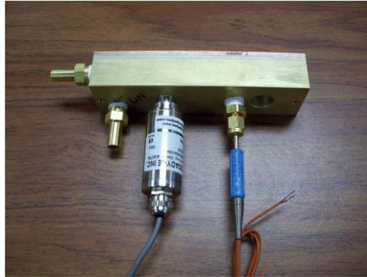
Figure 6: Liquid vapor Separator
