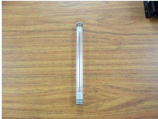
Figure 5: Bubble Pump Lift Tube
