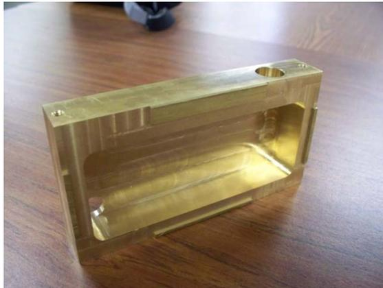
Figure 2: Cold Plate Cavity
