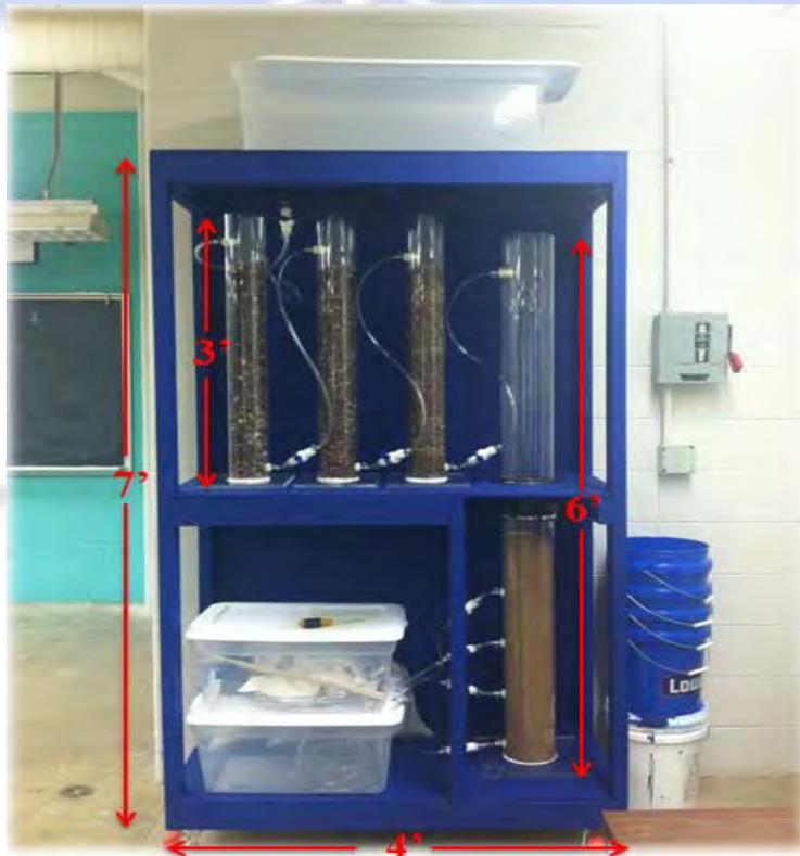
Figure 5: Final Design of SSF System
