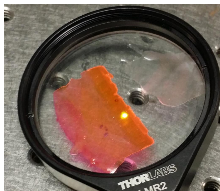
An example dye target (excited by a green laser) and the spectroscopy setup.
