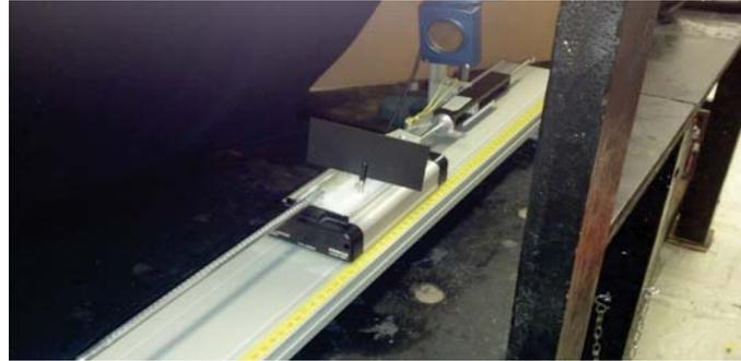
Data collection gives a clear look at the velocity before collision, and the velocity of both carts moving together after the collision.
