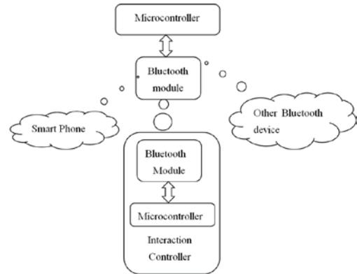
Fig.12. The communication system of the robotic fish
