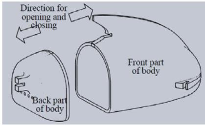
Fig.6. Two parts of the shell
