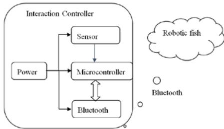
Fig. 13. Configuration of interactive controller
