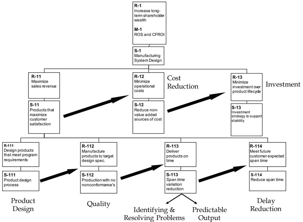
Fig. 2. Detailed decomposition of requirements to evaluate manufacturing system performance
