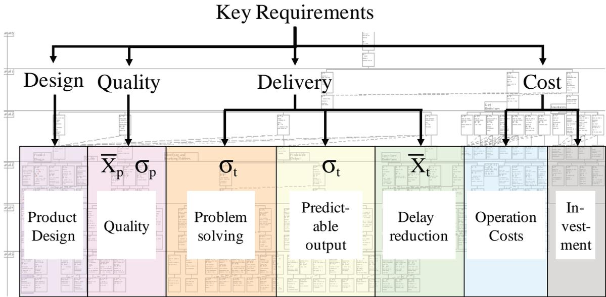
Fig. 1. Key requirements and design precedence of a path dependent manufacturing system
