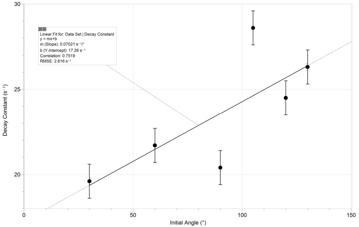
This is a graph of the best linear fit of the decay constant as a function of the initial angle  $\theta$ . The initial angle was calculated with respect to the resting position of the pendulum
