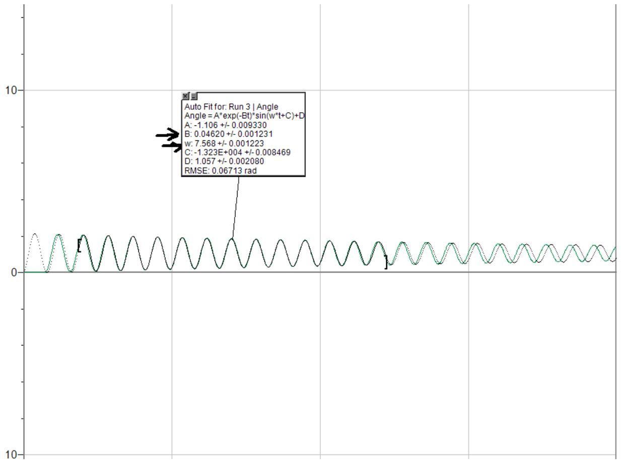
This graph shows that the data in tables 1 and 2 were calculated using a fit line for the behavior of a pendulum.
