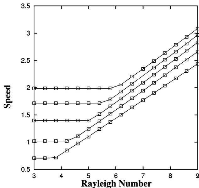
FIG. 2. Increase of speed near the onset of convection as a function of the Rayleigh number. The lines correspond to values of  $\mu = 1.0, 0.75, 0.5, 0.25,$  and  $0.0$  from top to bottom. The flow is for a viscous fluid.
