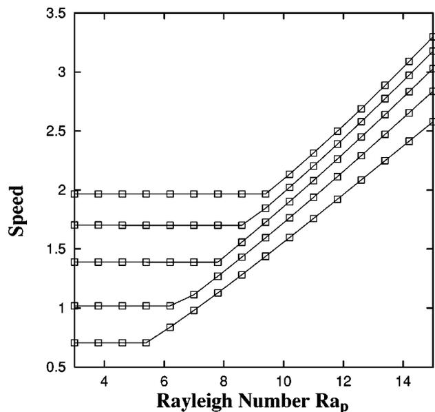
FIG. 1. Increase of speed near the onset of convection as a function of the Rayleigh number. The lines correspond to values of  $\mu = 1.0, 0.75, 0.5, 0.25,$  and  $0.0$  from top to bottom. The flow is for a fluid in porous media.
