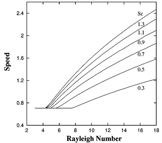
FIG. 7. The increase of speed as a function of Rayleigh number for different values of the Schmidt number. The width of the slab is equal to four. The flow is for a viscous fluid.
