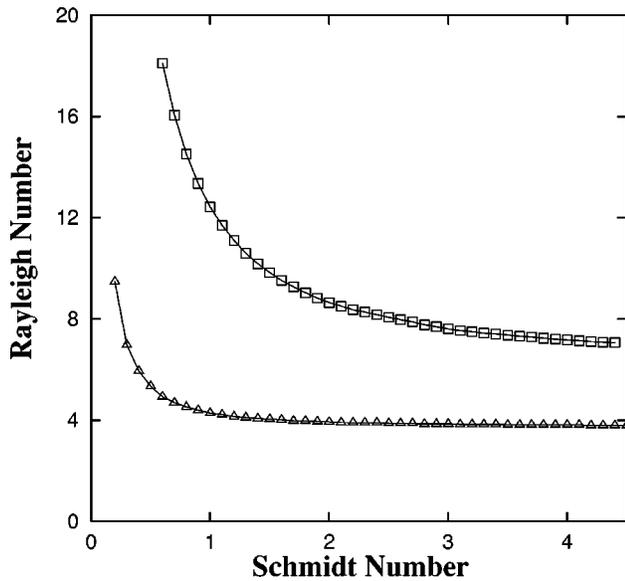
FIG. 6. The critical Rayleigh number as a function of the Schmidt number. The width of the slab is equal to four.
