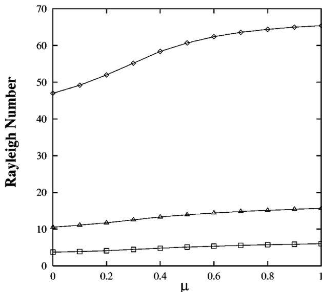
FIG. 4. The critical Rayleigh number as a function of mixing parameter  $\mu$ . The diamonds correspond to a fluid propagating in a slab of width two, the triangles for a width three, and the squares for a width four. The widths are in dimensionless units. The flow is for a viscous fluid.
