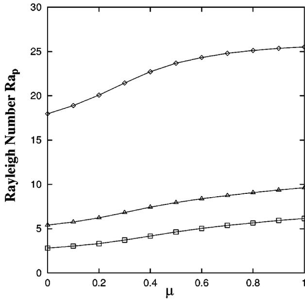
FIG. 3. The critical Rayleigh number as a function of mixing parameter  $\mu$ . The diamonds correspond to a fluid propagating in a slab of width two, the triangles for a width four, and the squares for a width six. The widths are in dimensionless units. The flow is for a fluid in porous media.
