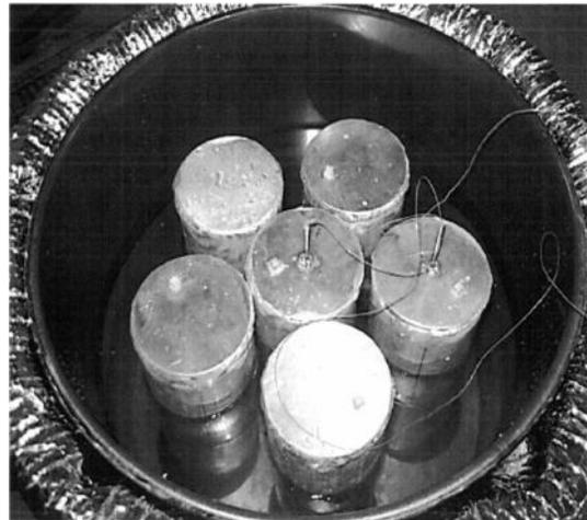
Fig. 4. Heat Exchangers inside the Water Reservoir
